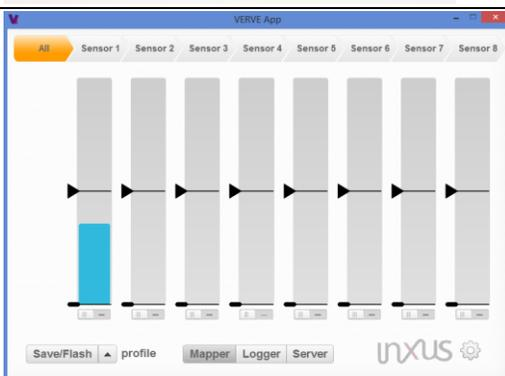
6. In the VERVE app, the blue bar shows you the response of the sensor. As you rotate the turn sensor left to right you will see the Sensor 1 bar move up and down.
