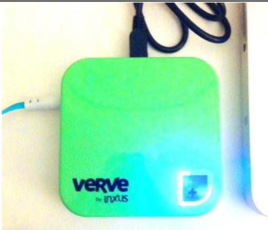
9. Press the black button on the VERVE 2; it should glow blue. This indicates that the VERVE 2 is in keyboard emulation mode. When your sensor value goes into an active zone, the keyboard action gets triggered.
