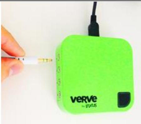
5. Plug the other end of the cable into port labeled **1** on the VERVE2 hub.
